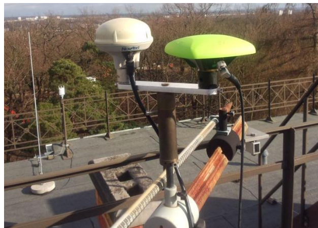
Figure 2.1 Experimental platform for single-frequency receiver validation
