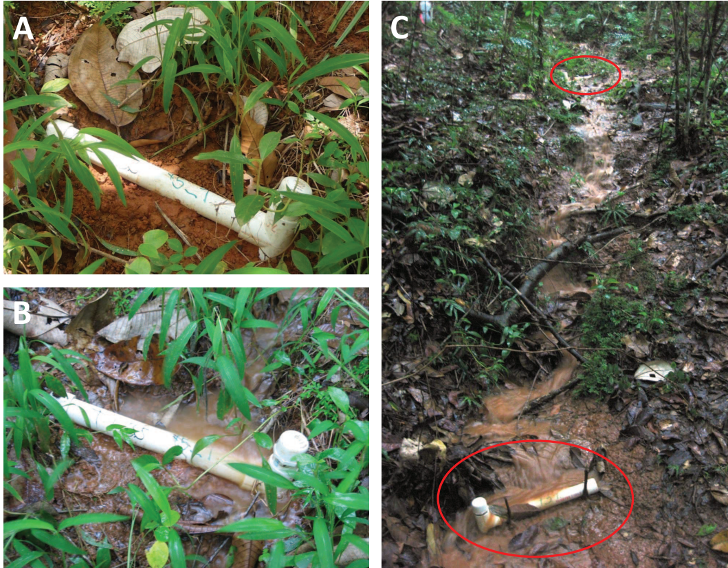
Figure 5.2: An overland flow detector (OFD) in dry (A) and wet (B) conditions. (C) shows connectivity in a flowline between two OFDs during a rainfall event.
