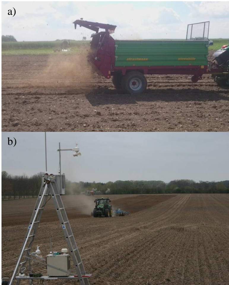
Fig. 1.5. Monitoring dust emissions downwind during a) manure application (Photo: © O. Biniash) and b) land preparation (Photo: © R. Funk).
