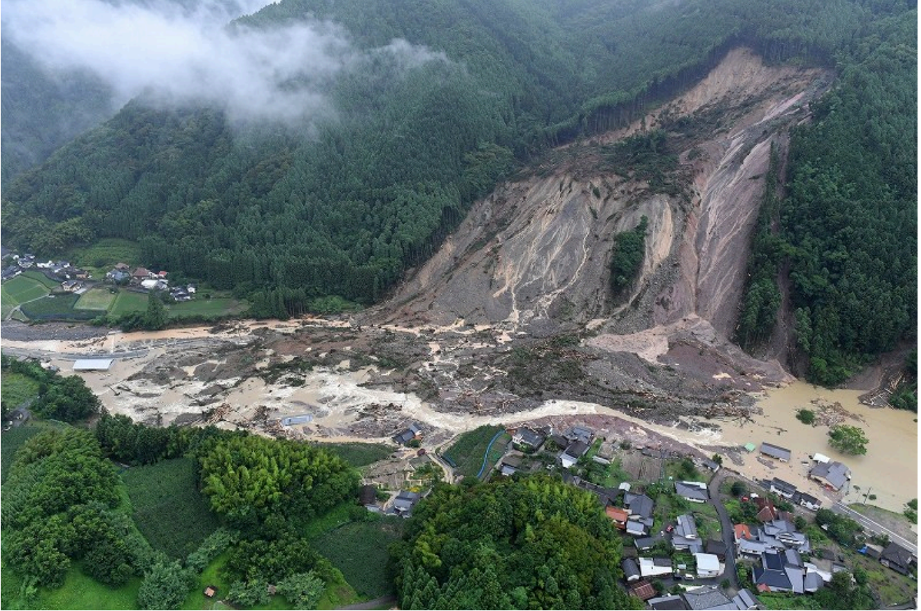
FIGURE 5.6: A landslide in Oita Prefecture, Japan at 11:33 on July 7, 2017, foot of which reached to the stream network during the 2017 Fukuoka floods (mainichi.jp, accessed August 6, 2018). It is likely that part of the slumped material is carried further downstream by the high waters.
