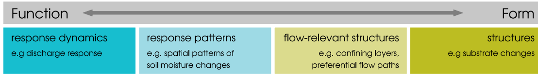
Figure 2.1: The concept of form and function applied to observations in hillslope hydrology. Four different categories which can be applied to data as well as the data sources.
