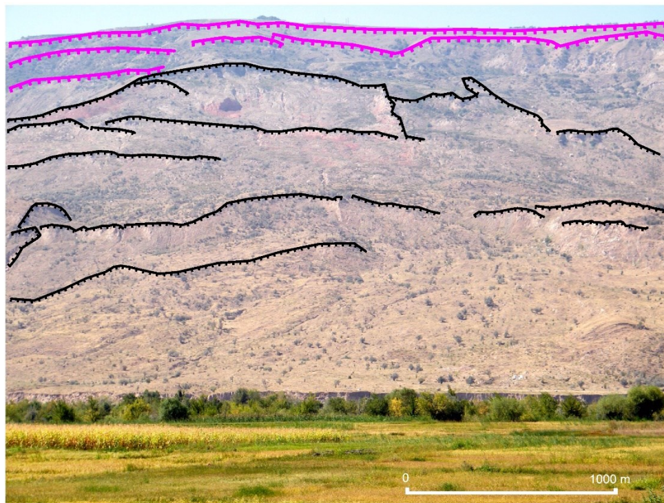
Figure 6. Mapped landslide complexes derived from optical remote sensing data and field observations. Perspective view of the eastern slope (Fig.4) overlaid by Rapid Eye imagery acquired on the 5th April 2011 (upper panel) and field photo (yellow box) taken on 11 September 2012 (lower panel). The individual landslide bodies are indicated by different colors, the main scarps are depicted in magenta and secondary scarps are depicted in black.
