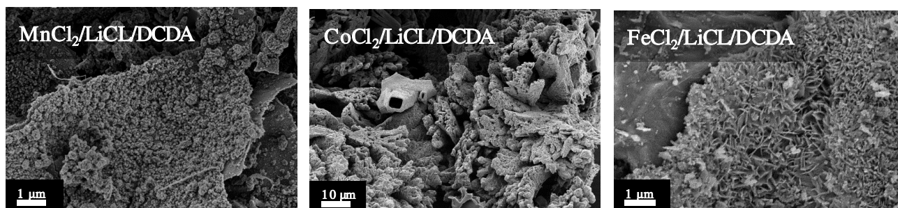
Figure S3: SEM images of \text{MnCl}_2 (1), \text{CoCl}_2 (1) and \text{FeCl}_2 (1) mixed with \text{LiCl} (2) / \text{DCDA} (0.5) and heated up to 800\text{ }^\circ\text{C} . The numbers in brackets display the molar ratio of the used compounds.
