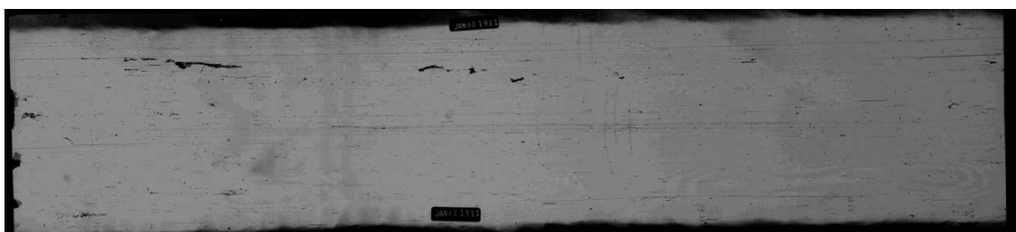
FIGURE B.1: Example of a bad quality seismogram which cannot be digitized. The record is from SLM seismic station (Wiechert instrument), both components are present on the record but not marked.
