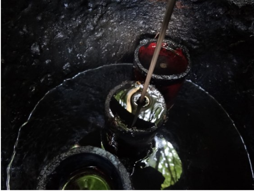
Fig. 1.13: Temperature logging in a 300-m-deep, narrow piezometric tube (9/02/2011).
