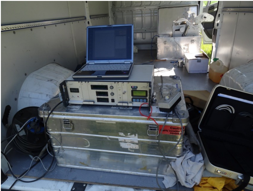
Fig. 1.14: Electronic control unit and computer for regulating logging speed, data recording and processing (9/02/2011).
