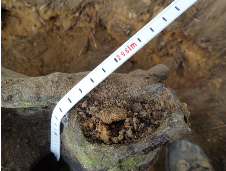
Fig. 1.11: Verification of the accessibility of the Mersch borehole with an electrical contact gauge by L. Schintgen and TS (7/15/2011).
