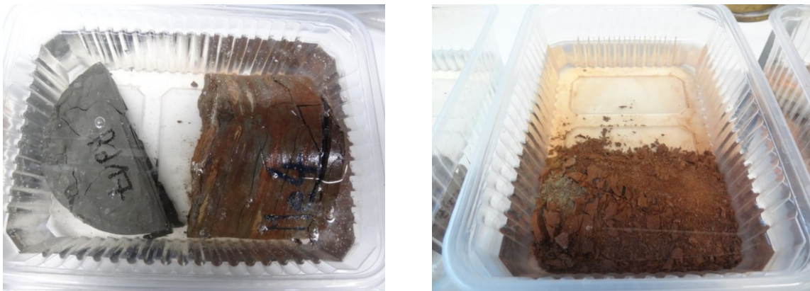
Fig 1.6: Example of claystone/marlstone samples reacting to water and being damaged.
