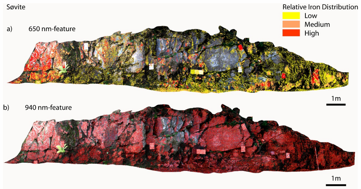
Figure 3.1.11: Thematic map of iron oxide showing the søvite outcrop. The classification was done using the MIFD. The underlying images were acquired with the HySpex imager (R, G, B color composite).
