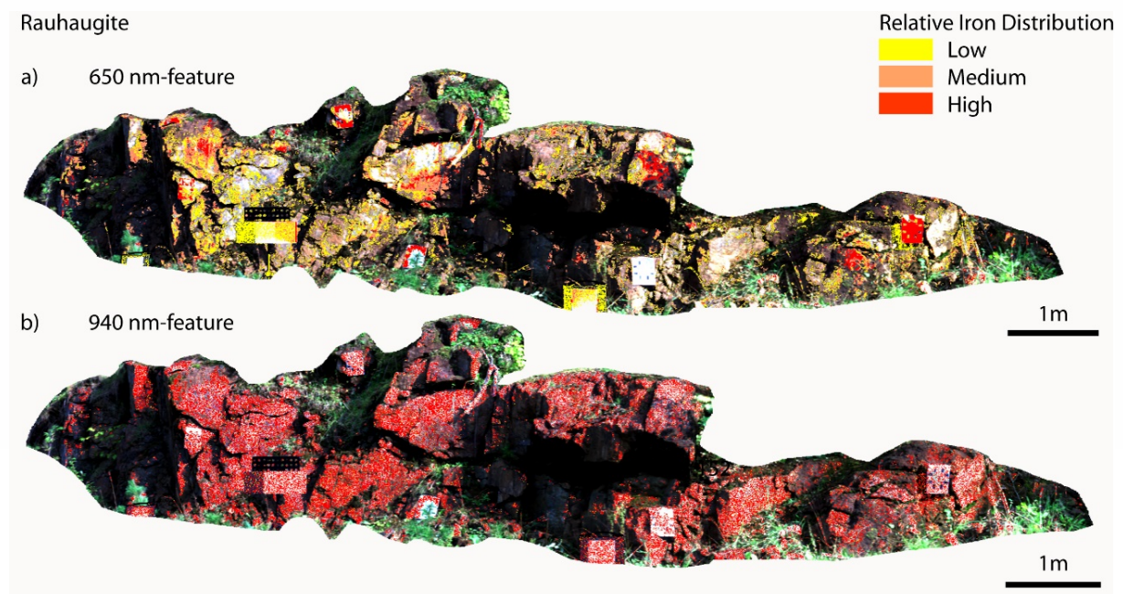
Figure 3.1.12: Thematic map of iron oxide showing the rauhaugite outcrop. The classification was done using the MIFD. The underlying images were acquired with the HySpex imager (R, G, B color composite).
