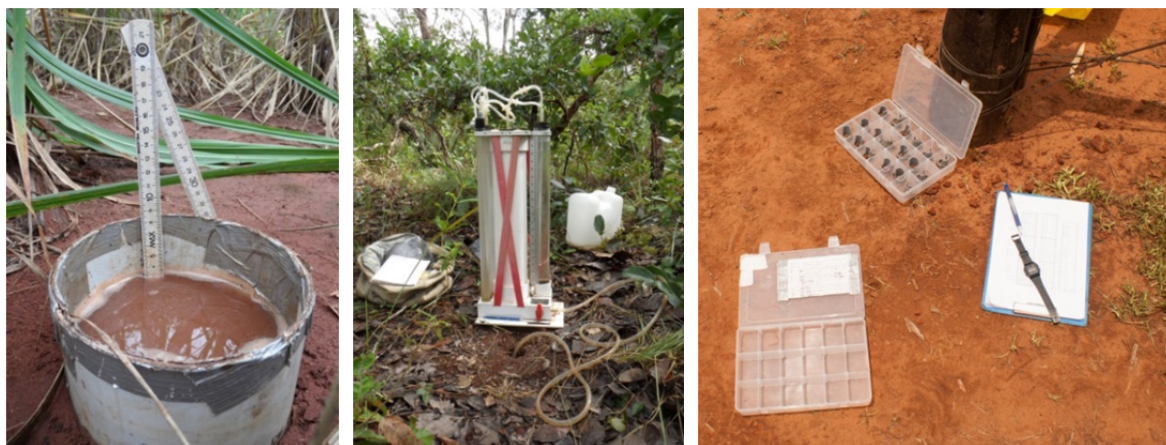
Figure 3-3. Ring infiltrometer, amoozometer and the Herrick test kit for determining aggregate stability.
