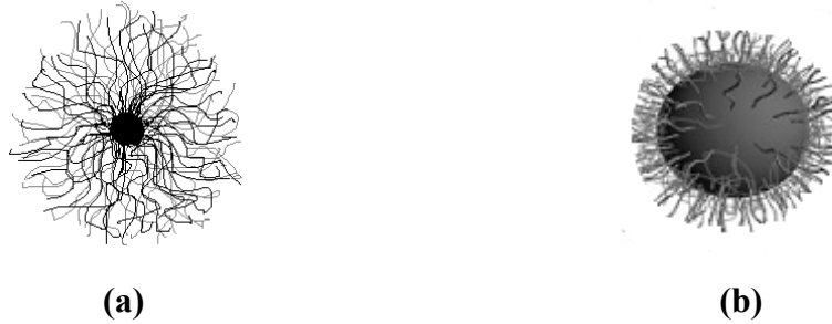
Figure 2.5: Schematic representation of (a) a hairy micelle and (b) a crew cut micelle.
