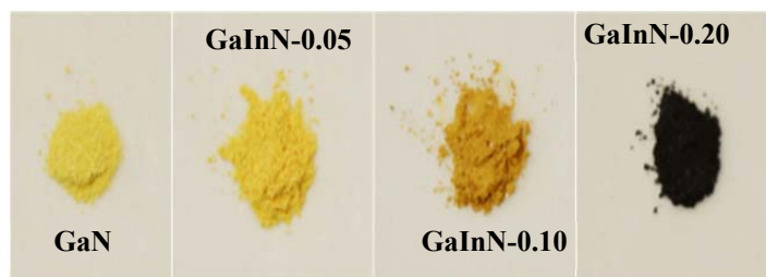
Figure 4.1.1.12. Gallium-Indium nitride samples prepared with R=5 and varying amount of In (table 9.3). The indium loading strongly affects the band gap of the final alloy and, as a consequence, different colours can be observed, from light yellow (colour of the pure GaN) to dark blue (colour of the pure InN).
