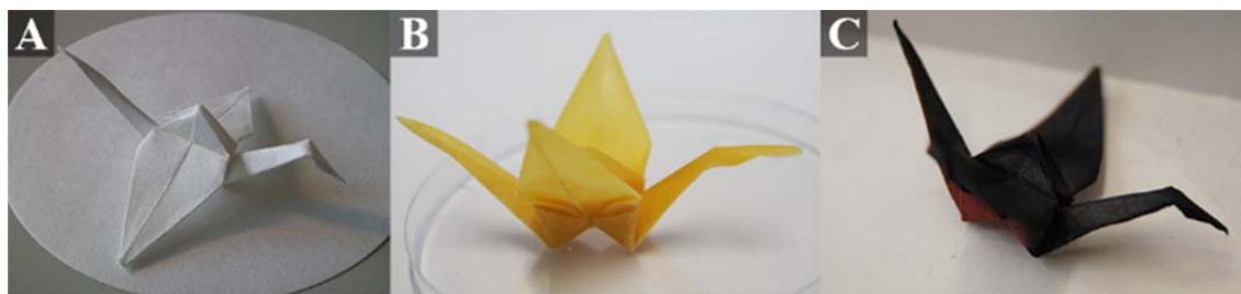
Figure 4.3.4. A filter paper folded as a “crane” (A) then soaked with the iron precursor solutions (B) and finally heat treated under \text{N}_2 flow up to 800^\circ\text{C} (C). Adapted with permission from reference [230] (© 2013 Wiley-VCH Verlag GmbH & Co. KGaA, Weinheim).
