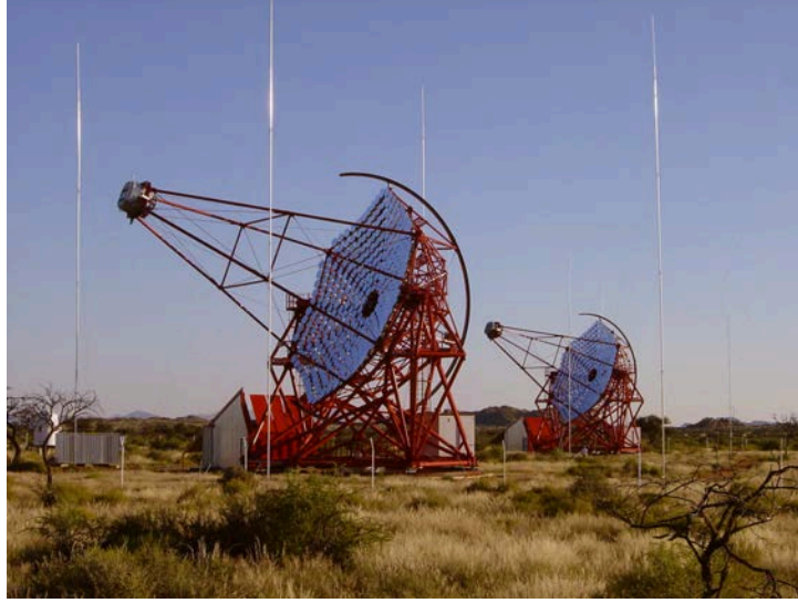
Figure 3.14.: Two of the H.E.S.S. 12 m telescopes, each with 382 mirror facets. Credit: H.E.S.S. collaboration.
