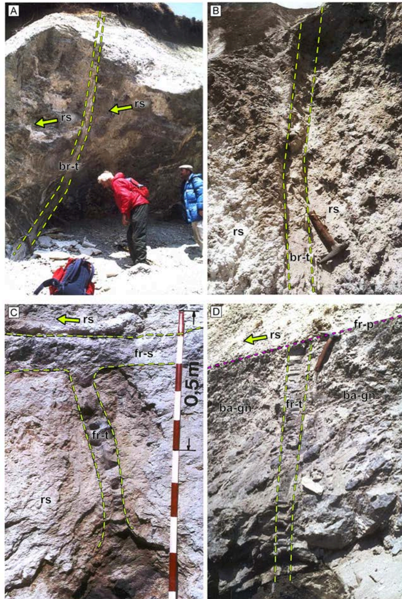
FIGURE A.4: Vertical tertiary shear planes composed of breccias (br-t) within rockslide mass (rs), composed of migmatites and leucogranites, Tsergo Ri rockslide, resulting from collision of the sliding mass with obstacles. Frictionite was found in the vertical breccia horizon in B). Vertical tertiary shear planes composed of frictionite (fr-t) within rockslide material (rs) C) and gneissic basement (ba-gn) D), Tsergo Ri rockslide. Field evidence suggests that these vertical planes are shearing planes, which have opened during sliding and into which frictionite has been injected during its creation along the associated primary shear plane (in D) and secondary shear plane (in C).
