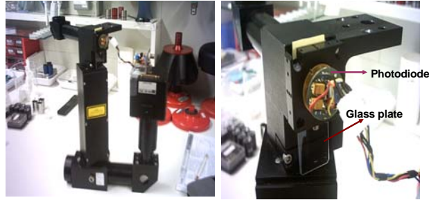
Fig.30 Photographs showing the fitting of the photodiode with the beam stop fitted to the optics. The photodiode with the beam stop was fitted in the optics path by gluing it on a glass plate and by removal of the components starting from the prism in XL-I optics(ref. fig. 5)
