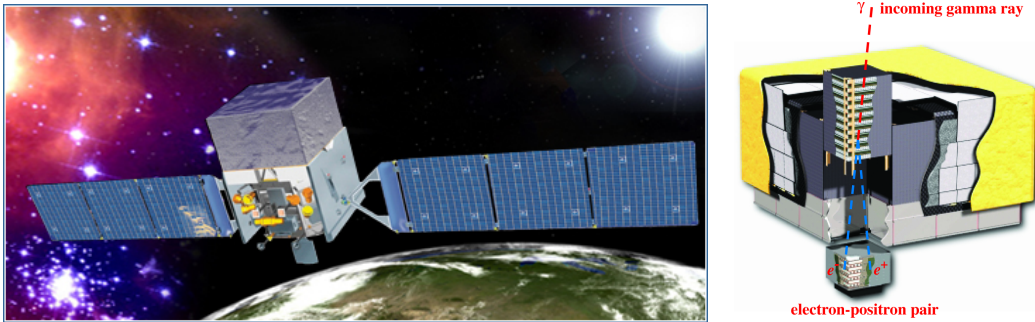
Figure 4.1.: Left: Artist impression of the Fermi Satellite. Right: A sketch of a vertical profile through the LAT, highlighting the most important subsystems. Further illustrated is the path of an incident HE \gamma -ray.
