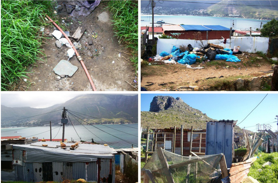
Figure 9: Infrastructure and services in the Hangberg informal settlement (informal water-connection, dumping station, electricity connections and sanitation facility) Source: Own photographs (2011)
