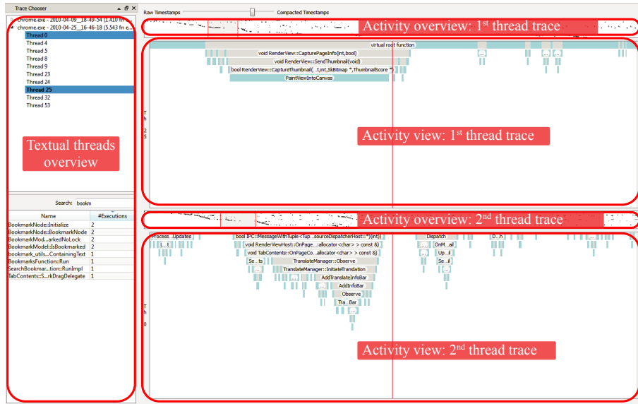
Figure 4.1: TRACEVIS user interface showing two thread traces.
