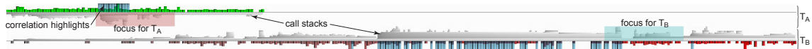
Figure 5.7: Overview visualization. The top and bottom parts show the match highlights and call stacks for the two compared traces, respectively.
