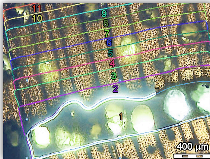
UV-laser dissection of a teak ( Tectona grandis ) cross-section (Author's picture: photograph taking during cutting process)
