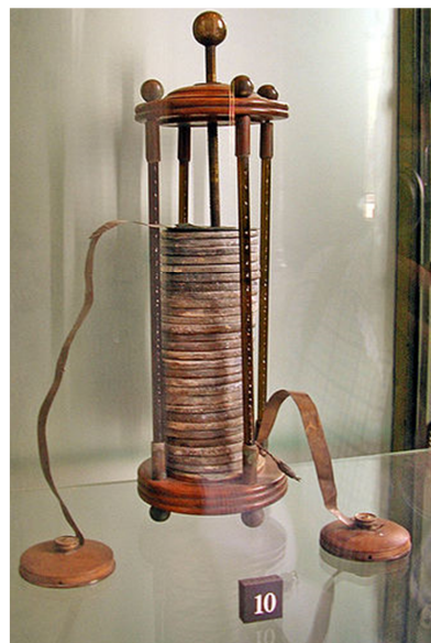
Fig. 22 Reconstruction of the voltaic pile with zinc and silver electrodes (GNU license)
