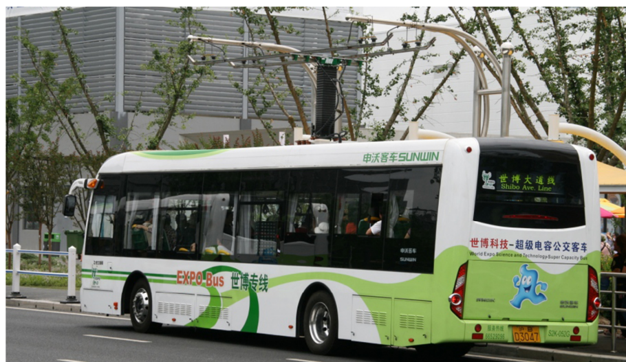
Fig. 9 EV Bus (capabus) currently tested in Shanghai; large onboard supercapacitors are used as power source; SCs are charged at bus stops and by break energy recuperation (GNU license)
