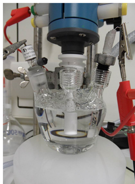
Fig. 21 Left: Schematic representation of the 3-electrode test setup with working (WE), reference (RE) and counter electrode (CE) and electrolytic resistance between working/reference ( R_{WR} ) and working/counter ( R_{WC} )
