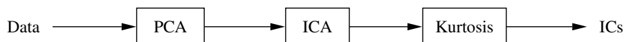
Figure 4.2: The proposed ICA procedure. First, the data set is reduced by PCA thereby maintaining all of the relevant variances. ICA is applied to this reduced data set and the extracted independent components are ranked by their kurtosis value to obtain components that are sub-Gaussian distributed.
