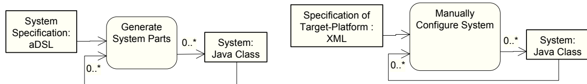
Figure 6.10.: Example for two activities, where it cannot be excluded that the hard changeability concern unexpected loss of content is affected. Notation based on UML activity diagrams [156].
