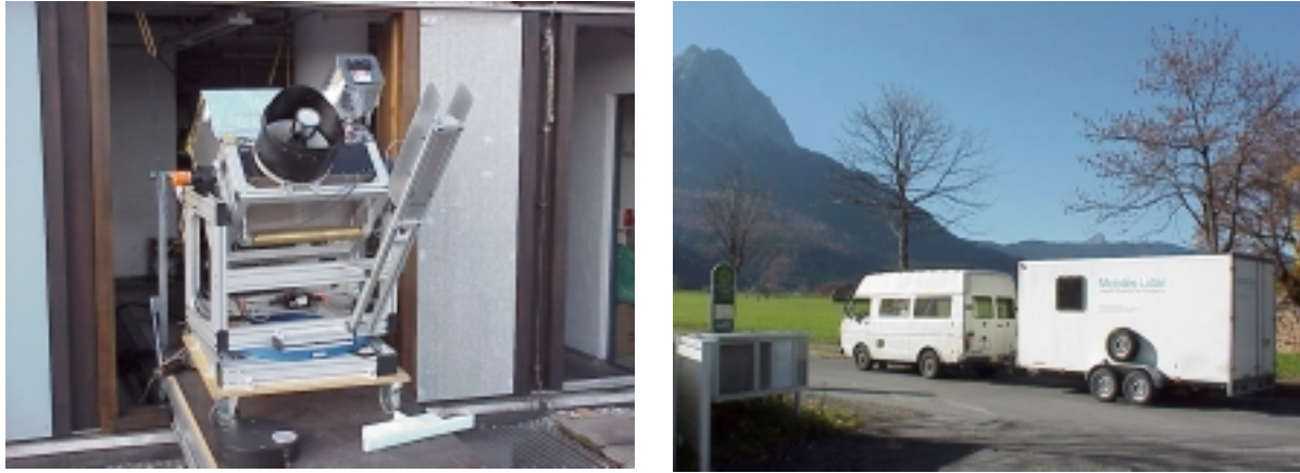
Fig. 1: Lidar device of the Ludwig-Maximilians-Universität München, see Wiegner 2000, for environmental monitoring by remote sensing
