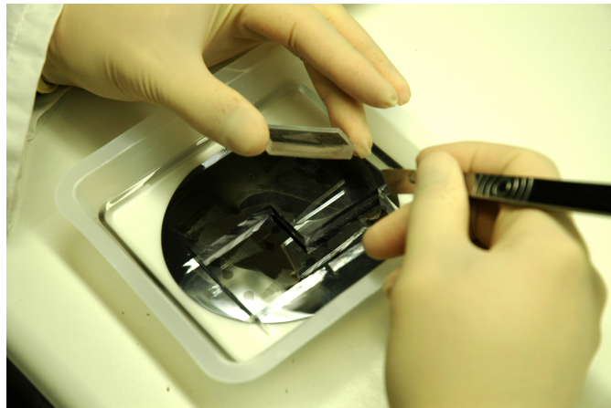
Fig. 4.5: Preparation of a microfluidic experiment: a channel made from PDMS has been cut out using a scalpel. This corresponds to the transition from step one to step two in figure 4.4. The PDMS block is a negative replica of the structure printed on the wafer. After punching holes for the fluid inlets, plasma cleaning and sealing with a coverslip, the microchannel is ready for use.
