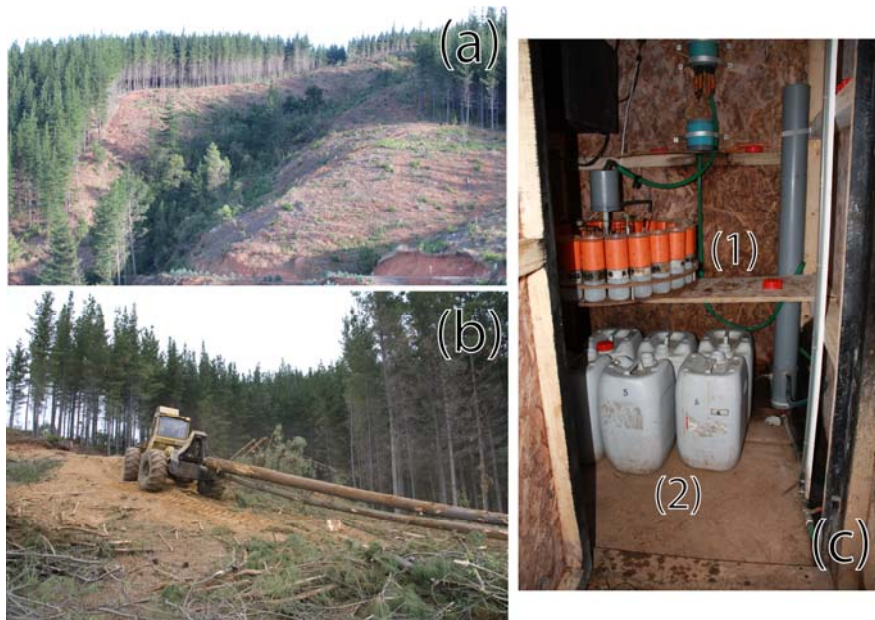
Figure 4.2. Pictures showing the experimental catchments, the logging procedure and the suspended sediment monitoring devices. (a) Rainy season logged watershed (watershed #3) in the subsequent dry season (March 2010); (b) Skidder dragging logged stems uphill to the next landing in watershed #3; (c) Custom-built sediment sampling system: (1) Horizontal rotating table used to sample suspended sediment on event-base; (2) Recipient used to collect bulk sample of suspended sediment on weekly base.
