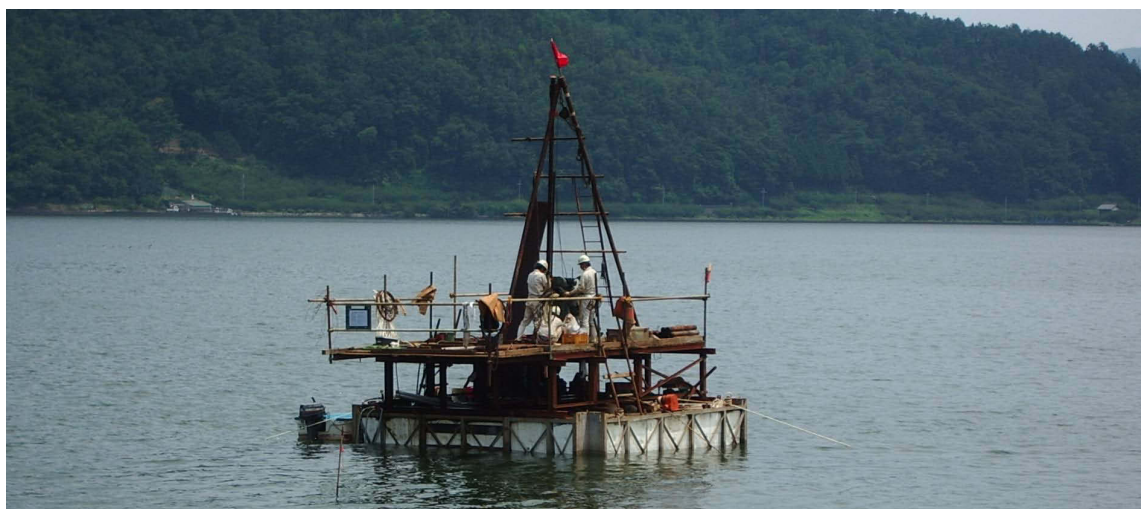
Figure I.3.: The drilling platform used for the Lake Suigetsu sediment coring campaign conducted in the summer of 2006.
