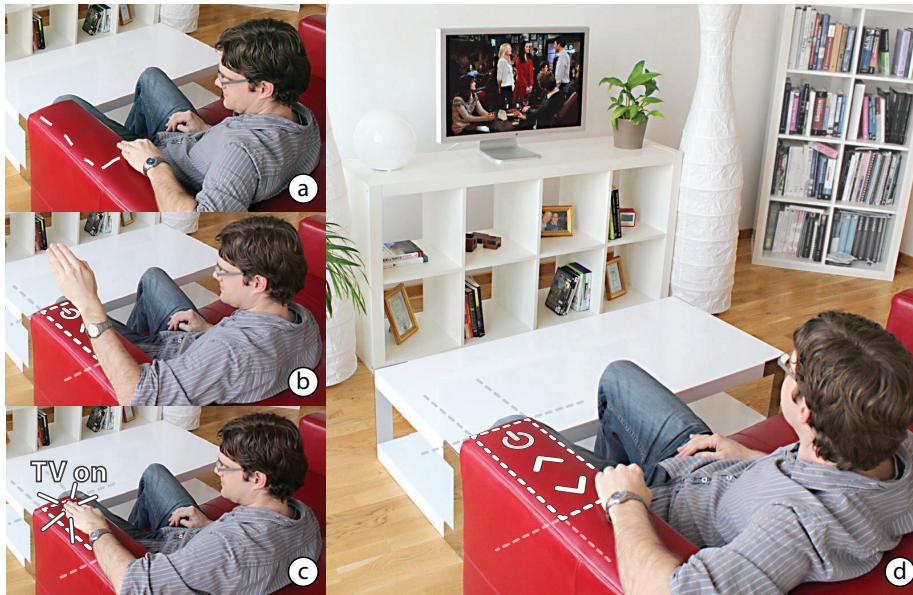
Figure 4.16: The principles of Imaginary Interfaces could also be applied to situations other than mobile interaction. Here a user is interacting with a draw-your-own imaginary interface on the couch in his living room. (a) He first draws a rectangle on the arm rest to tell the system where he wants the (b) remote control to be placed. (c) Then he can turn on the TV by touching the location associated with the ON button and (d) watch TV without looking for the remote control.
