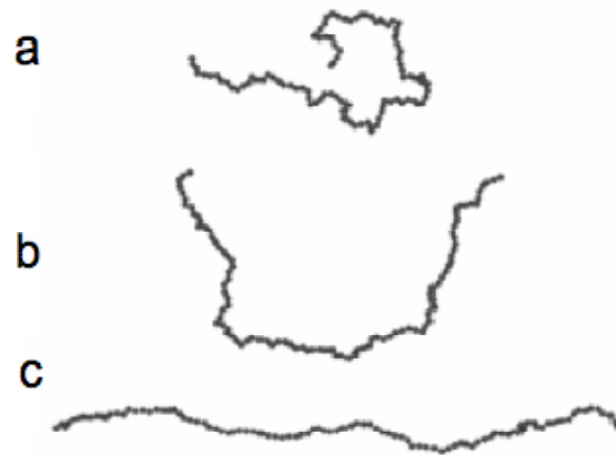
Figure 2-2: Monte-Carlo Simulations of the influence of different salt concentrations on the polyelectrolyte conformation. The bare persistence length was kept constant while the Debye screening length was chosen to give an electrostatic contribution to the persistence length which is on the order of the monomer size (a), (b) several monomers, (c) the contour length of the polymer [10].
