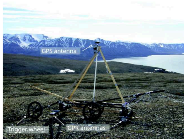
Figure D.3.: A photo showing the GPR antenna cart on a relatively even section of the field site on top of the Wordiekammen plateau (view toward south). We used additional wooden constructions to stabilize the GPR antennas and the differential GPS antenna, given the harsh field conditions.
