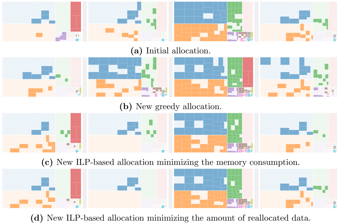
Figure 6.14.: Visualization of allocated data for changing workload: TPC-DS with K = 4 nodes.
