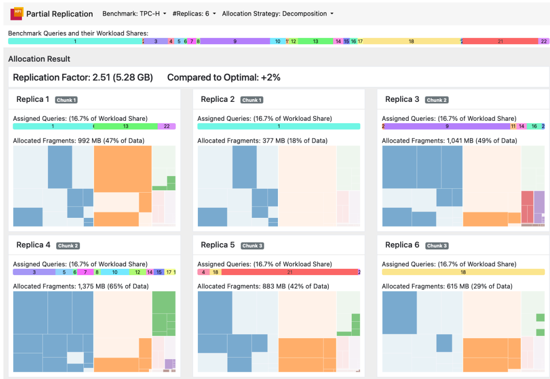
Figure 6.1.: The application screenshot shows an allocation of our decomposition heuristic for a cluster with six nodes running the TPC-H workload. [101]
