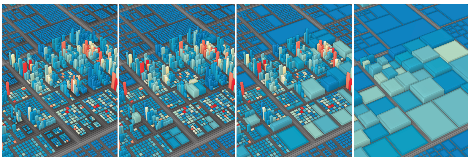
Figure 4.4: Stepwise simplification of a treemap using aggregation, ranging from little aggregation (left) to strong aggregation (right). The LoD is controlled using DoI scores and, as shown here, is based on the tree level.
