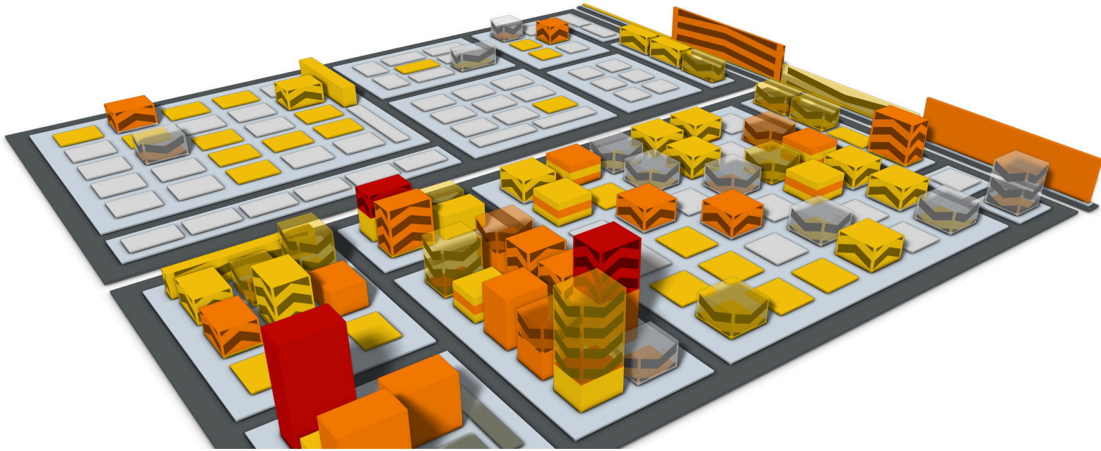
Figure 3.17: Example of a 3D-embedded treemap using in-situ templates for a simultaneous two-state mapping to height and color. The implementation of templates can be challenging. For example, the display for a drop in height (cf. I_{12} in Figure 3.18) uses procedural arrow textures [L21] and order-independent, stochastic transparency [68].
