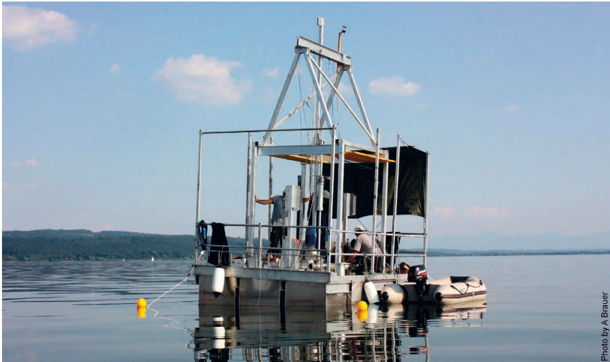
Figure 1.4. Sediment coring on Lake Ammersee in summer 2010 using a modified UWITEC piston corer installed on a stationary float.
