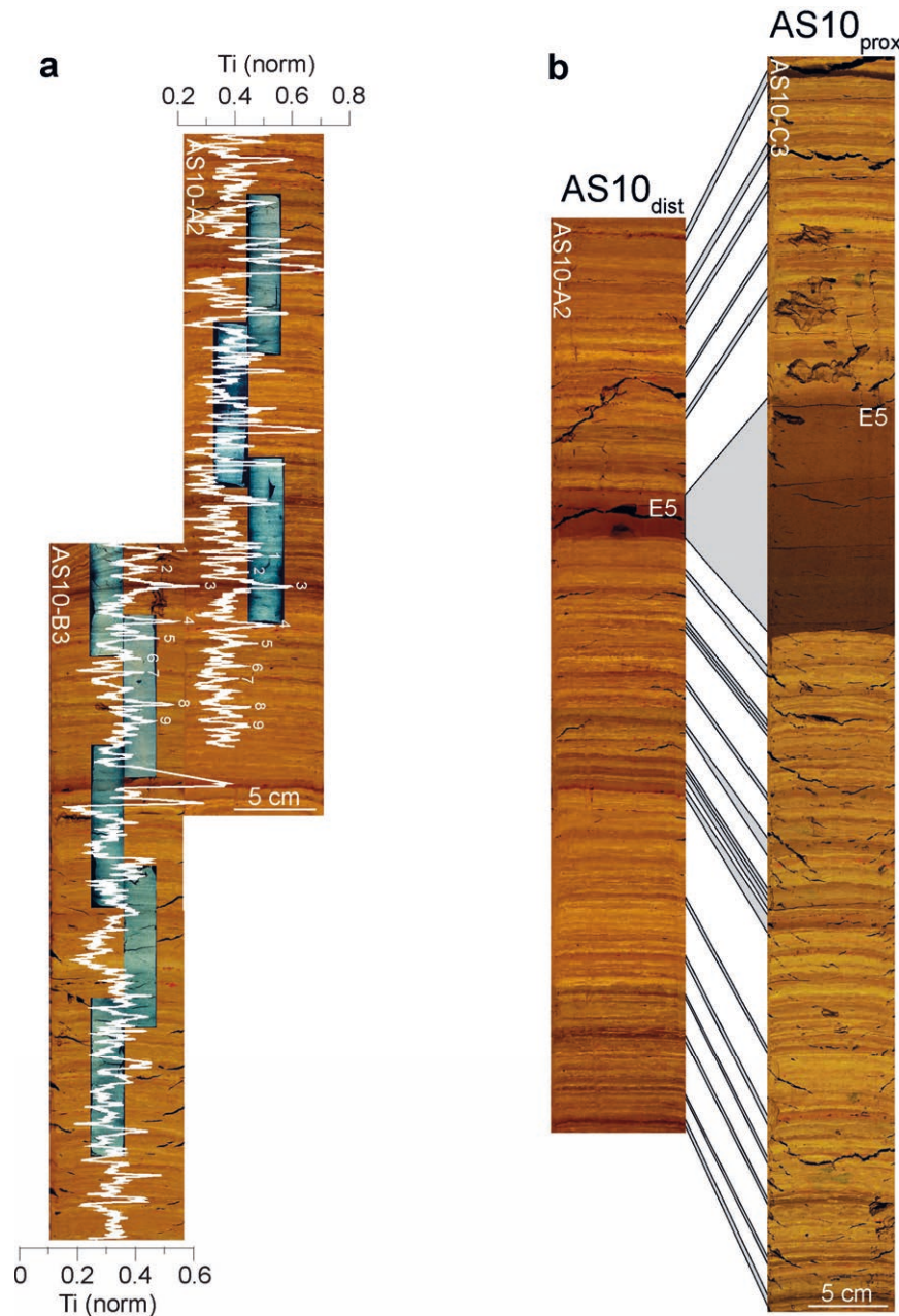
Figure 3.4. Correlation of sediment profiles. (a) Core-to-core correlation of parallel core segments using lithological marker layers and element profiles (Ti norm). (b) Intra-basin correlation of sediment profiles AS10 prox and AS10 dist based on macroscopic lithological marker layers.
