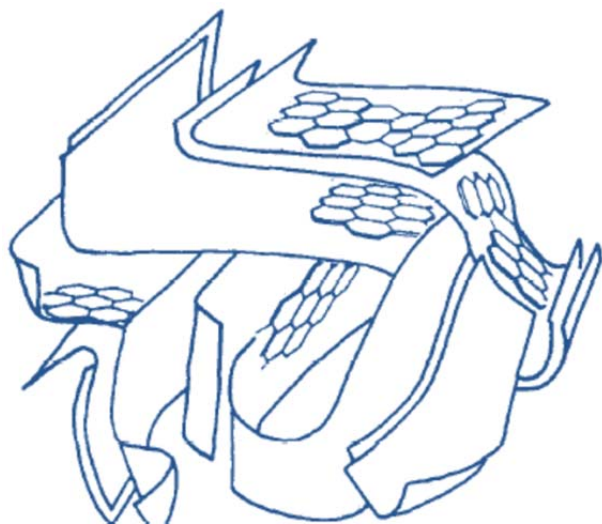
Figure 1-10 Schematic illustration of the structure motives occurring in activated carbon. Adapted from reference 97. [97]
