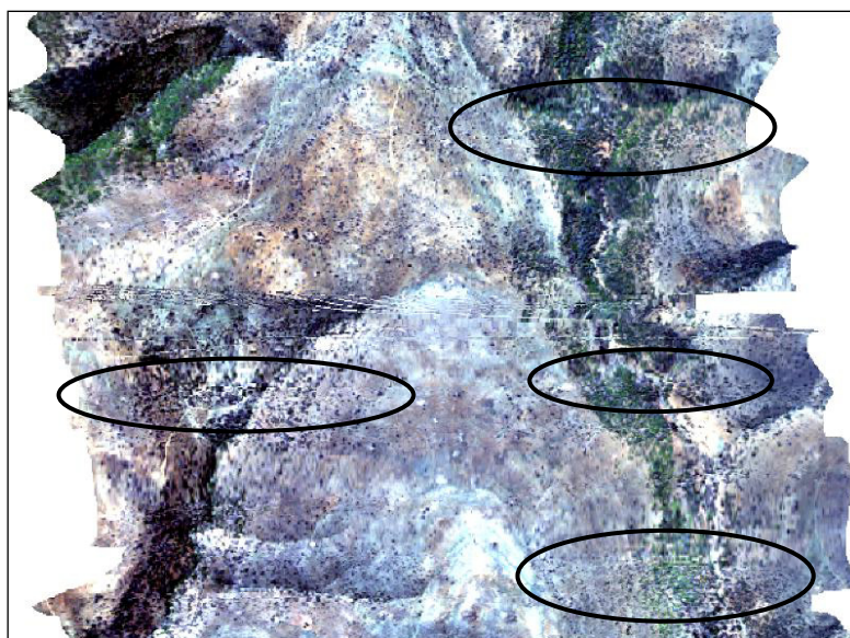
Figure B-3: One large and some smaller artifacts remain in the orthorectified imagery. Detailed view of flight line 3 as true color image (with R: 640 nm, G: 549 nm, B: 456 nm).
