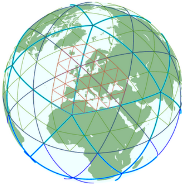
Figure 4.1: Illustration of the grid construction procedure. The original spherical icosahedron is shown in blue, denoted as R1B00 following the nomenclature described in the text. In this example, the initial division ( n=2 ; dark blue), followed by one edge bisection ( k=1 ) yields an R2B01 grid (red lines), (Prill et al., 2020).
