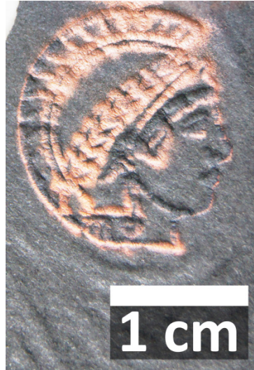
Figure 63: Photo of deposited copper on the printed Minerva structure. The resulting deposition is not flawless but can none the less serve as a proof-of-concept.
