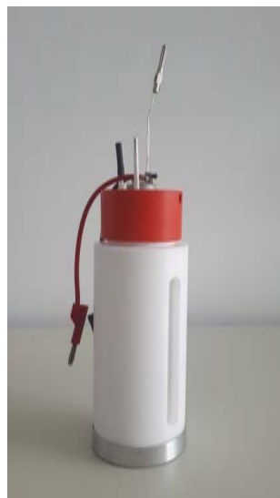
Figure 2.4: Inner container of the etching cell.
