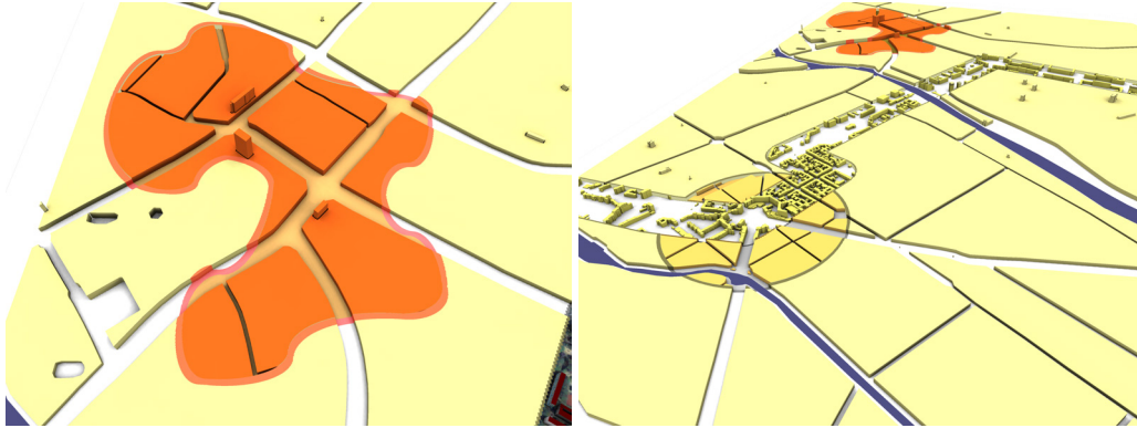
Figure 3.21: Generalization lenses allow the combination of different LOA representations in one image. Therefore, different areas of interest to the user can be highlighted as focus regions. Lenses of focus regions may have arbitrary shape (left) and overlap themselves. An example is the highlighted course of a route that crosses a highlighted plaza (right). The definitive version of these images can be found at (Glander and Döllner, 2009), ©Elsevier.
