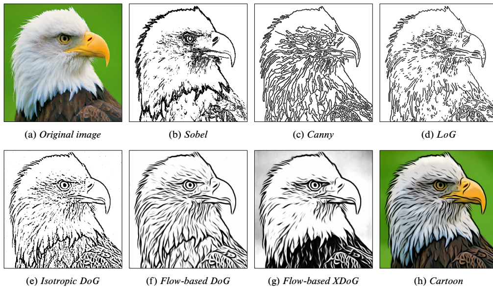
Figure 4.3: Example showing the output of different edge detection and stylization methods. (a) The original image. (b) The globally thresholded gradient magnitude of the Sobel filter. (c) The output of the Canny edge detector [Can86]. (d) Zero-crossing of the Laplacian of Gaussian [MH80]. (e) The thresholded DoG as proposed in Winnemöller et al. [WOG06]. (f) The thresholded output of the separable implementation of the flow-based DoG. (g) The flow-based DoG with XDoG thresholding. The image is pre-processed with a bilateral filter to suppress noise. (h) Cartoon-style abstraction generated with bilateral and flow-based DoG filters using the generalized cartoon pipeline.
