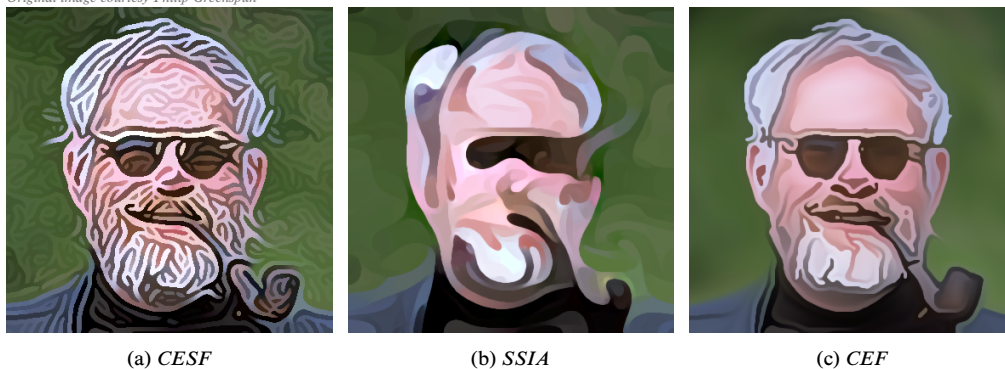
Figure 6.19: Limit cases. (a) Coherence-enhancing shock filter [Wei03] with 50 iterations. (b) Shape-simplifying image abstraction [KL08] with 50 CMCF iterations. (c) Proposed method with 50 iterations.
