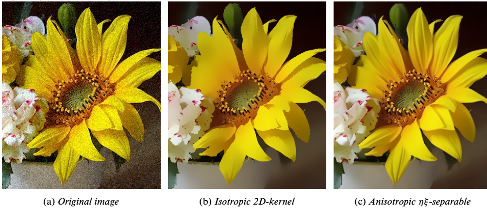
Figure 3.7: Adapting the separable implementation of the bilateral filter to the local structure enables the enhancement of image structures. (a) Original low quality image. (b) Bilateral filter: \sigma_d = 6 , \sigma_r = 8\% . (c) Orientation-aligned bilateral filter with linear sampling: \rho = 4 , \sigma_{d,g} = 3 , \sigma_{r,g} = 2\% , \sigma_{d,t} = 8 , \sigma_{r,t} = 10\% . In both cases 5 iterations were performed.
