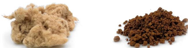
Cellulose (left) and lignin (right) from beech wood after REM treatment
