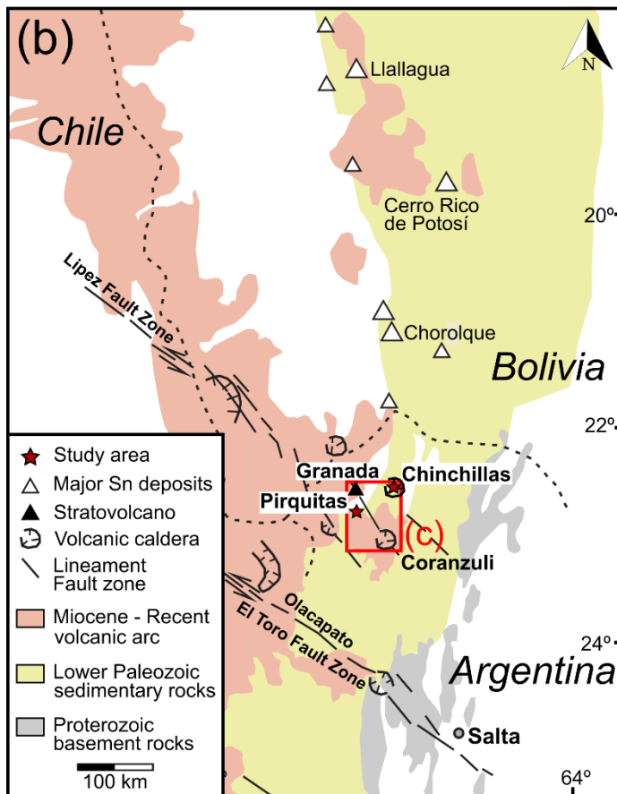
Figure 30 Map of the southern sector of the Central Andean Tin Belt with the location of the Piriquitas deposit in the southernmost part. Miocene porphyry and subvolcanic intrusions, caldera structures, major WNW-trending lineaments, and fault zones as well as the dominant host rock lithologies are shown (modified from Passamani et al. 2020).
