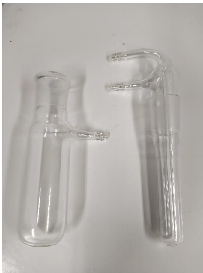
Figure S3.1. Custom reactor for scaled-up photocatalytic reaction with a gas adapter (left) and its internal cold finger condenser (right).
