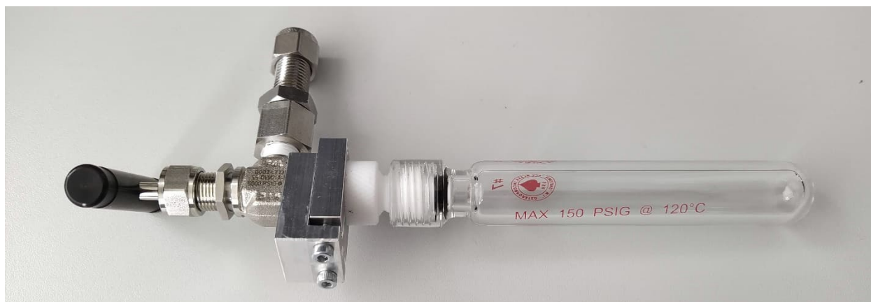
Figure S3.2. Custom reactor for photocatalytic experiments under oxygen pressure.
