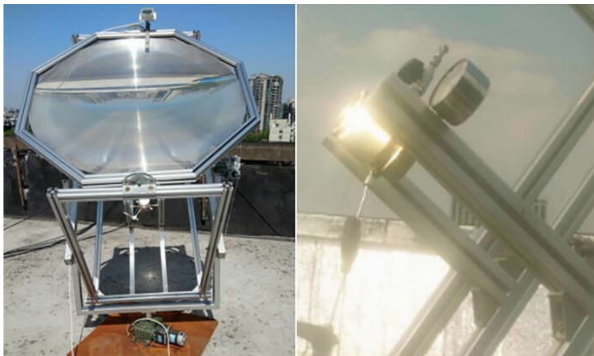
Figure 1.4. Solar concentrator setup for batch photocatalytic CO 2 reduction (left) and close-up of its reaction chamber (right). Reprinted with permission from ref (52) . Copyright 2021 AIP Publishing.
