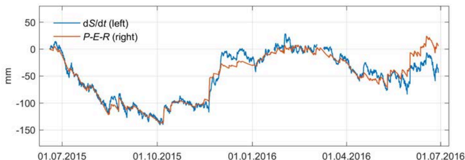
Figure 3.10: Time series of water storage at Wettzell (as a deviation from the initial storage value at the beginning of the study period, arbitrarily set to 0), with the measured iGrav006 gravity-based storage time series (blue line) (left side of Eq.3.3) and the optimized storage time series (red line) after optimization following the right side of the water balance equation (Eq.3.3).
