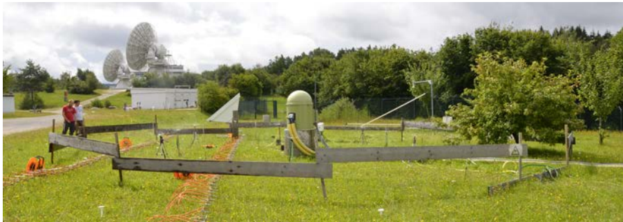
Figure 4.3: Setup of the sprinkling experiment at Wettzell Observatory (Bavaria, Germany), with an iGrav gravimeter in its field enclosure (green dome, center), sprinkling units on tripods and electrode profiles for electrical resistivity monitoring (orange).
