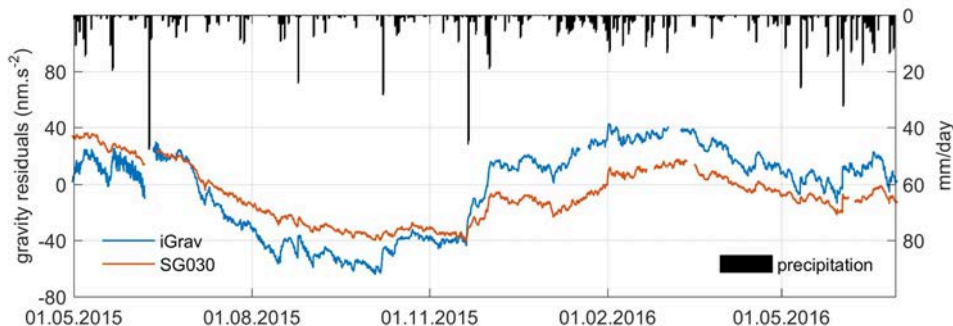
Figure 3.3: Time series of gravity residuals of iGrav006 in the field enclosure and of SG030 in the observatory building, and daily precipitation rates (from top and right axis) at the Observatory Wettzell.
