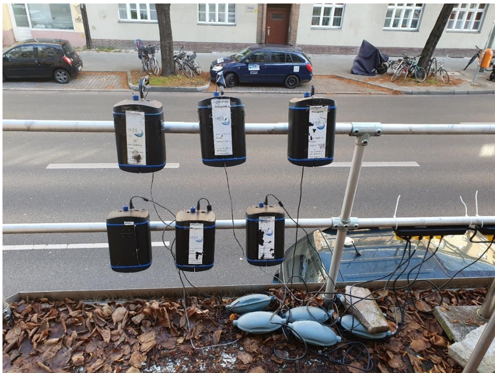
Figure 3.S-2 Set-up of the co-location of the Zephyrs at BLUME station MC 117 (Schildhornstrasse). A similar set-up was used at MC 174 (Frankfurter Allee) during the co-locations on Frankfurter Allee. An inlet to the right of frame draws air into the station for the reference instruments to use.
