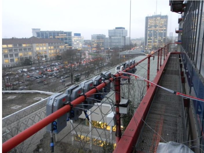
Figure 2-3 Set-up of the co-location of the prototype Zephyrs with reference instruments on the 6 th floor of the Mathematics building. The grey units are the Zephyrs, and the two inlet tubes connect to the reference devices located inside the office.
