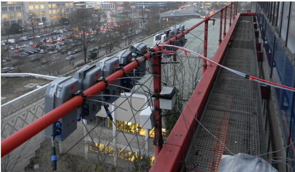
Figure 3.S-1 Set-up of the co-location of the Zephyrs with reference instruments on the 6 th floor of the mathematics building. The grey units are the Zephyrs, and the two inlet tubes bring air to the reference devices located inside the office.
