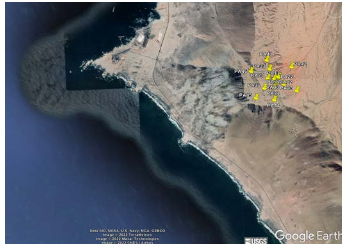
Figure 4.9: Screenshot of the array in Google Earth. The yellow pins stand for the PESO stations. The picture highlights the cliff escarpment. The shoreline orientation is in agreement with the beamforming results in which the noise strikes the array from a south-west direction.
