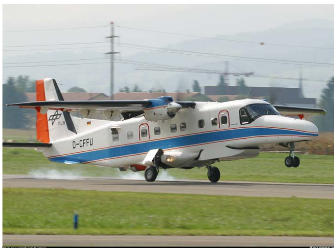
Figure 69: DLR's airborne E-SAR system on board a Dornier Do 228-212 aircraft [23].
