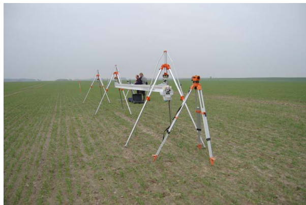
Figure 57: CESBIO-ESA LASER profiler with field campaign settings [23].
