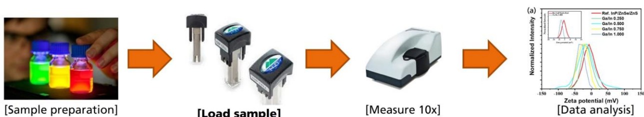
Figure 75. Schematic representation of the zeta potential measurement workflow using colloidal QDs.
