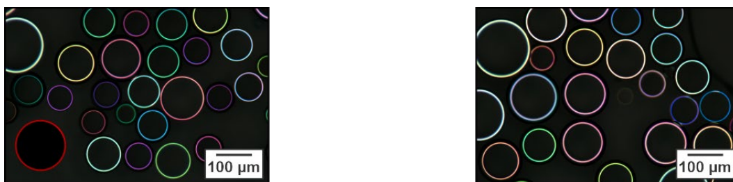
Figure 91. Reflectance optical micrographs of complex emulsion droplets showing how the color emanates from near the contact line and varies with droplet diameter.
