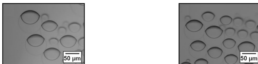
Figure 67. Side-view images of the ammonium complexation control experiments. Raising of the pH-value to 13 by adding sodium hydroxide (left) and presence of 2-[2-(3-aminopropoxy)ethoxy]ethan-1-ol (PEG-NH 2 ) (right) did not change the initial droplet morphology.
