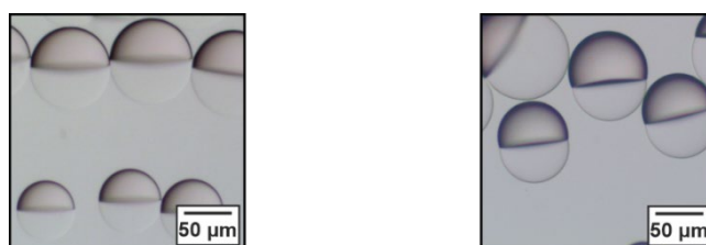
Figure 22. Side-view micrographs of hexane- (left) and octane-perfluorohexane Janus droplets (right) prepared in a surfactant solution containing 0.5 wt.% SDS and 1.5 wt.% Zonyl. The higher interfacial tension between octane and PFH leads to a slight elongation of the droplets in vertical direction.
