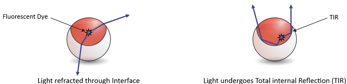
Figure 16. Illustration of 2D-ray diagrams of fluorescent light emitted in the high index HC phase of side-viewed droplets. Most of the emitted light will be refracted through the droplet interfaces (left), however some of the light emitted near the internal interface can undergo TIR (right). This light will most likely leave the droplet through the HC/W interface.
