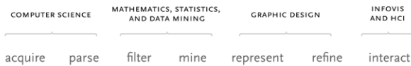
Figure 31: Ben Fry’s seven-step process from the acquisition of data to the interaction within the visualization interface 29
